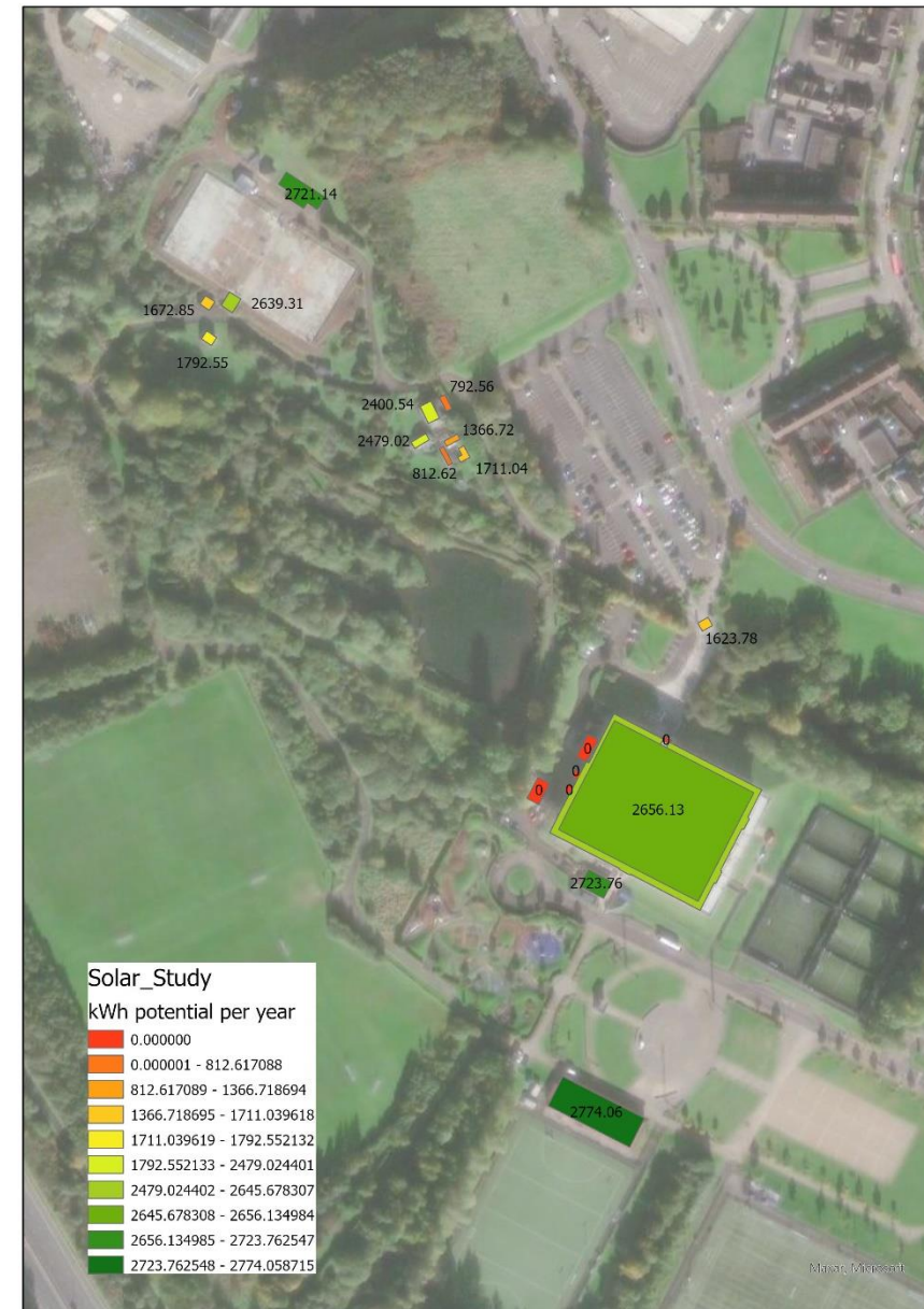
Fig. 1: Aerial view of Valley Park – buildings kWh potential if fitted with solar panels indicated by colour
